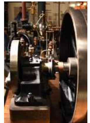
Porter-Allen high-speed steam engine popular late 1800s to early 1900s
